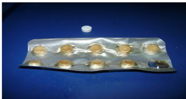
Fig. 4. Deformation of blister of MN ODTs (F2) after storage at 50°C for 2 months
